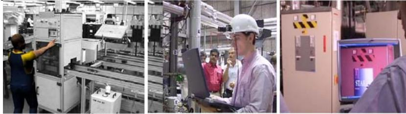
**Fig. 1.** First and second pictures from left: a virtual human demonstrates the use of a real machine (offline test requiring two machines). Third and fourth testing the real-time tracking with basic rendering in a factory (one machine).
