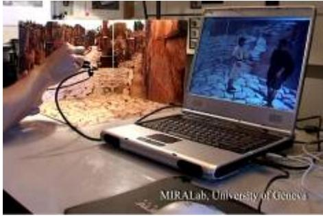
Figure 8 Lab ‘maquette’ controlled AR tests. For optimum flexibility and tests the camera is detached from the HMD and moved freely within the ‘tracked area’ augmenting it with virtual characters (laptop monitor)
