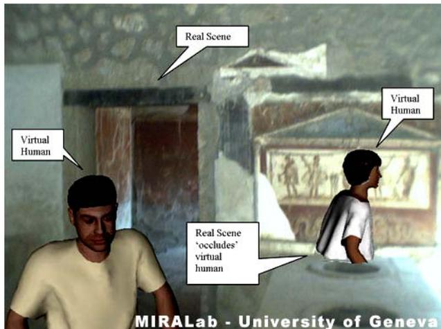
Fig. 7 Real-time virtual Pompeian characters in the real site of the Pompeian thermopolium. Note the use of geometry 'occluders' that allow part of the real scene to occlude part of the virtual human
