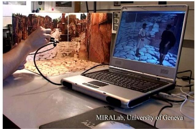
Fig. 3. Lab ‘maquette’ controlled AR tests. For optimum flexibility and tests the camera is detached from the HMD and moved freely within the ‘tracked area’ augmenting it with virtual characters (laptop monitor)
