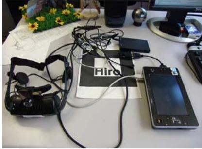
Figure 6. A wearable UMPC with the i-glasses HMD, battery pack and usb webcam.
